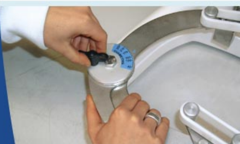
Beakers clamping (patented system)
