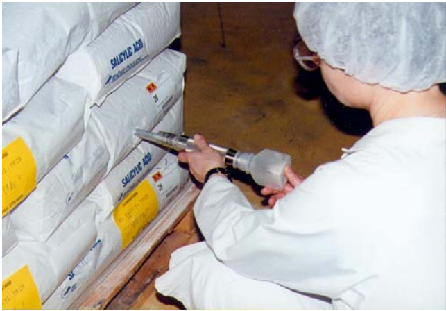
Solid pointed tip to penetrate easily into the sack contents.
